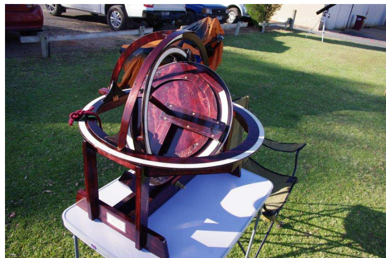
Above - ASV member built this beautifully crafted device which converts longitude & latitude (coordinate from a star chart) to Right-Ascension & Declination (degrees from north & degrees above the horizon) ... This is the second that Norman has built.
