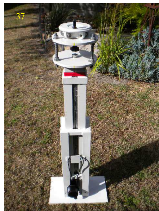
37. Troy has also built an electric lift pier for the Observatory, which allows him to reach the eyepiece, for those times when the eyepiece is in a hard to use position... Is also very handy when an object is low on the horizon. The pier carries his EQ6 mount.
